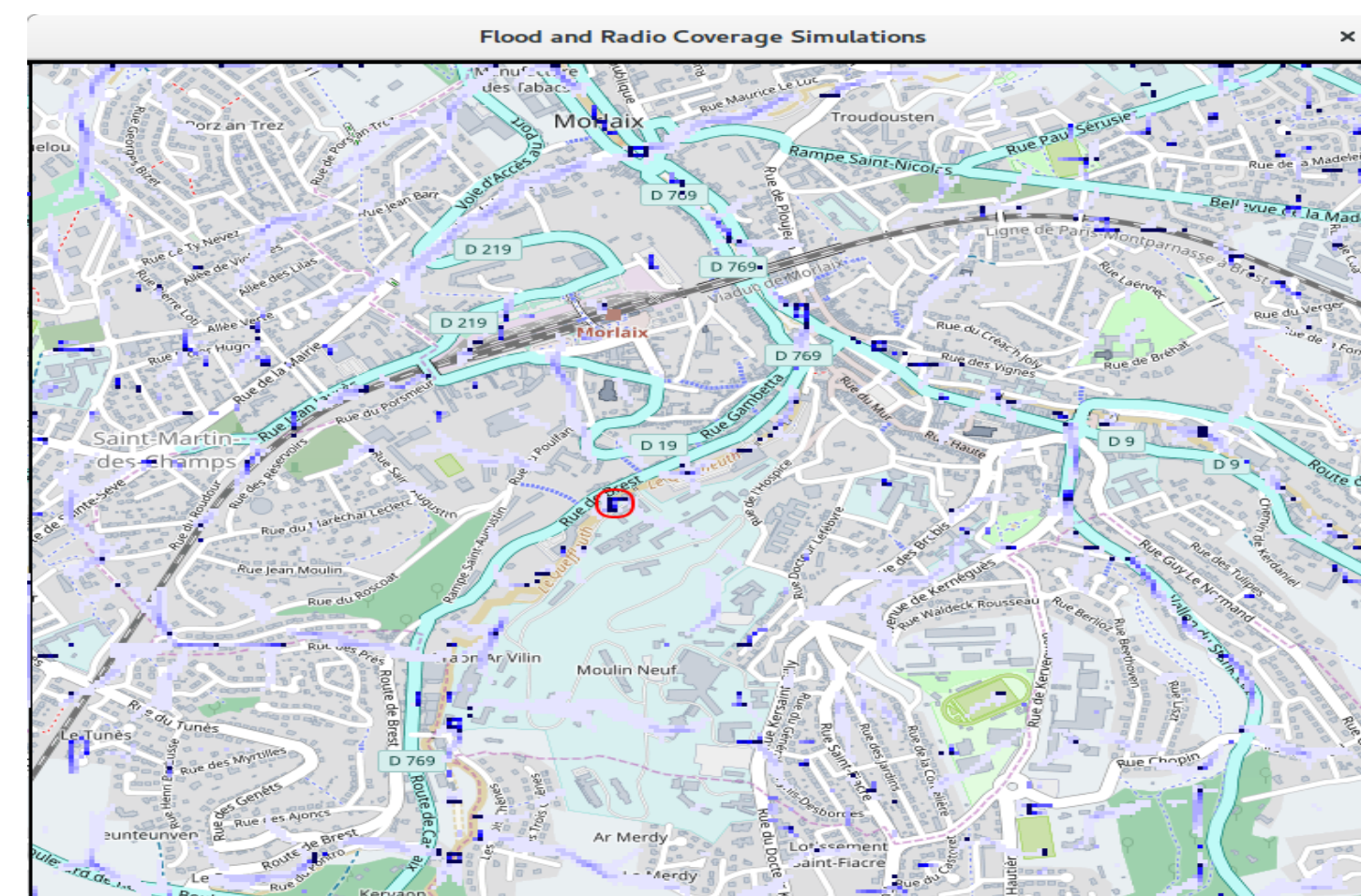
Fig 9. Morlaix (France) Simulation (58275 cells, 3 x 3 km, rainfall: 60cm) by GPUs with thousands of CUDA cores.
